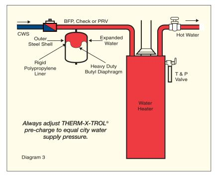
If your Plumbing Code requires a Backflow Preventer, Check Valve or Pressure Reducing Valve... You Need a THERM-X-TROL® on Every Job!
